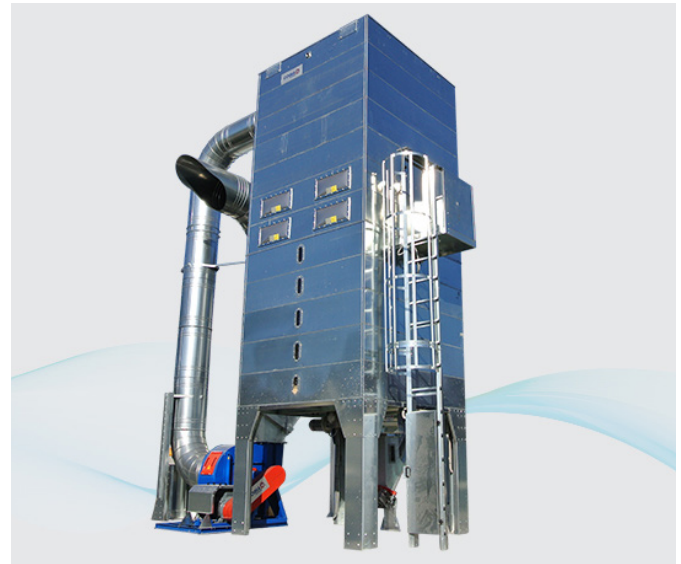
MVD-4 Mini-Silo Dust Collector featuring Explosion Vents and Silo Viewing Windows
