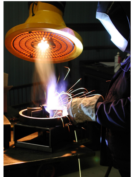
The Wing arm can be offered with built-in light, start/stop switch, manual or motorized damper.
